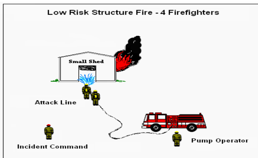
FIGURE 4-1: Low-Risk Response-Exterior Fire Attack
